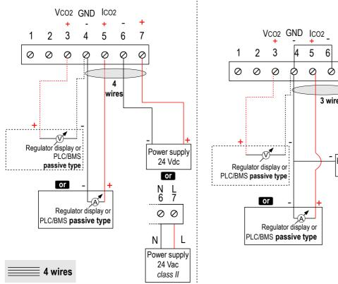
To make a 3-wire connection, before powering up the transmitter, please connect the output ground to the input ground. See drawing below.
